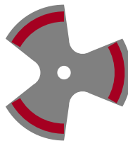
Fig. 5: Schematic front view of the chopper rotor of SPHERES. The red bands indicate the mosaic crystals that deflect the incident beam towards the monochromator.
