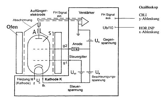
Figure 4: Circuit diagram for the Franck-Hertz tube.
