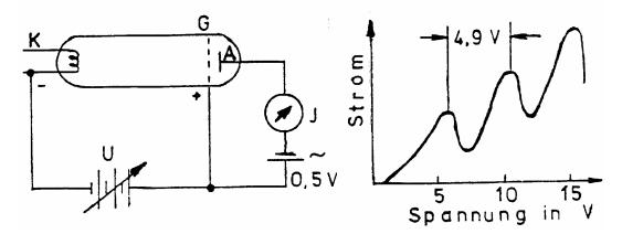
Figure 2: The Franck-Hertz experiment: a) Principle of the arrangemen; b) Current-voltage characteristic. Strom = current; Spannung = voltage.
