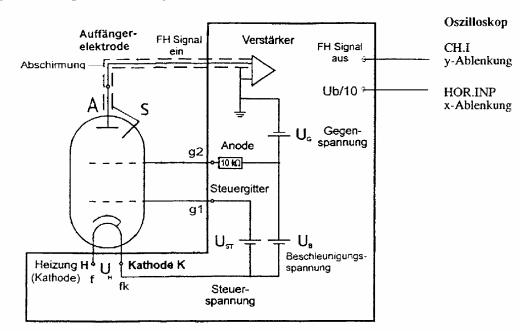
Figure 6: Experimental arrangement for neon.
